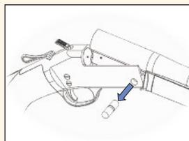
**2)** Remove the pivot pin by tapping it out with a 3/8" diameter or smaller wooden, brass, or plastic dowel or rod. This can be done from either direction.
