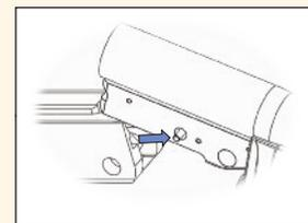
**3)** Remove the barrel assembly from the receiver assembly. The ejector/extractor release pin needs to pass cleanly through the slots in either side of the receiver. To reassemble, reverse these steps, making sure that you check for proper functioning of the action, hammer, and trigger mechanisms prior to loading and firing.
